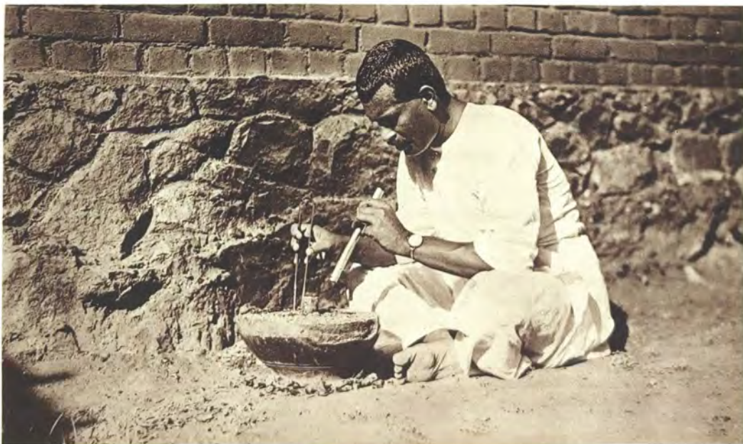
With the tongs in one hand and the blow pipe in the other, watching intently as he sits “a refiner and purifier.”
