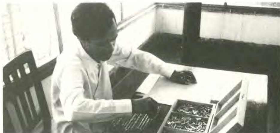
Joel Ahmed setting up Braille type for printing
